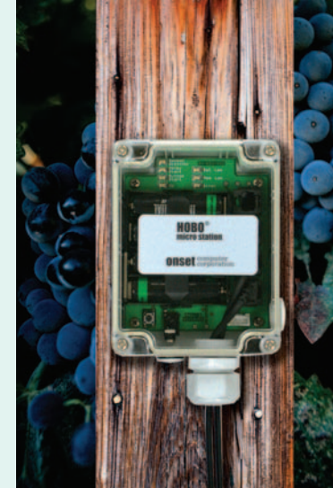
The HOBO Micro Station's small size is perfect for microclimate monitoring.
