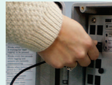
Expanding or reconfiguring the HOBO Weather Station or HOBO Micro Station is as simple as plugging in, or unplugging, smart sensors.
