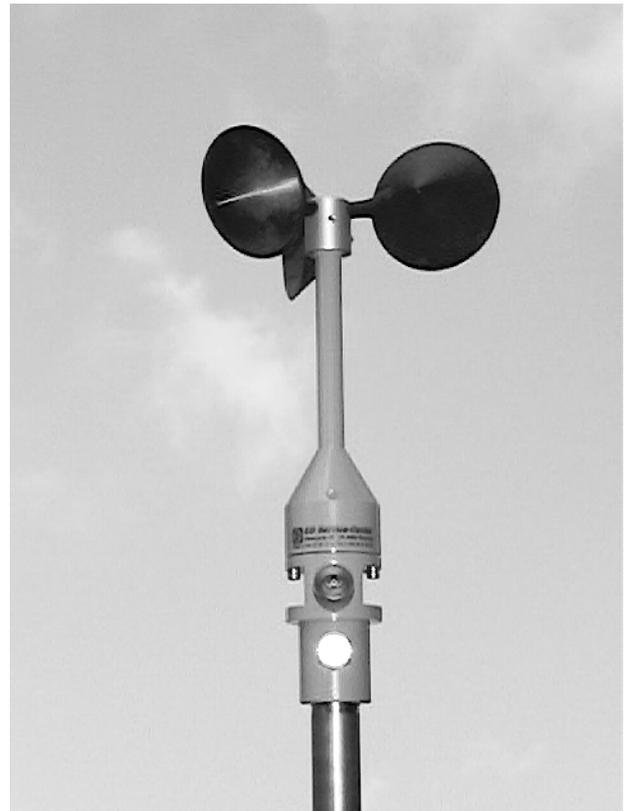
The ED-260-I Transmitter Module is used for signal generation in the ED Cup Anemometer. This module measures the time-period used for the anemometers shutter to complete one cycle. The ED 260-I generates a current-output by an high-performance current-source.
